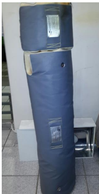
Figure 6. Barrel extruder insulation jacket.
